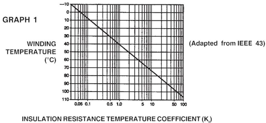
(3) Insulation resistance readings must not drop below the value indicated by the following formula:
