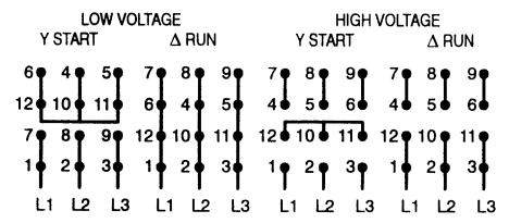
FULL VOLTAGE ACROSS THE LINE START AND RUN ON A CONNECTIONS. ALSO SUITABLE FOR START ON Y, RUN ON  $\Delta$ .
