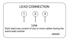
To reverse direction of rotation interchange connections L1 and L2. Each lead may be comprised of one or more cables. Each cable will be marked with the appropriate lead number.
