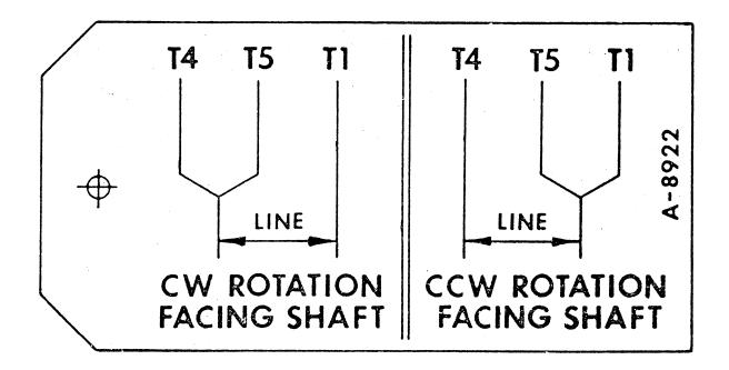
To reverse direction of rotation, interchange leads T1 & T4. Each lead may have one or more cables comprising that lead. In such case, each cable will be marked with the appropriate lead number.
