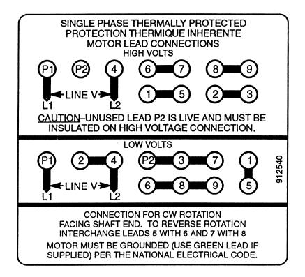
CW Rotation facing shaft. To reverse direction of rotation, interchange lead 5 with 6 and lead 7 with 8 for CCW Rotation. Each lead may have one or more cables comprising that lead. In such case, each cable will be marked with the appropriate lead number.
