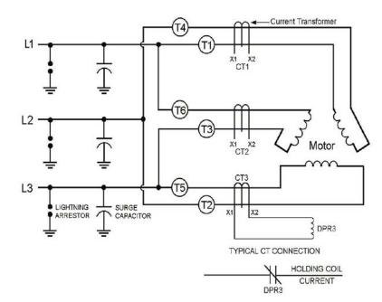
Delta Connected, Single Winding
