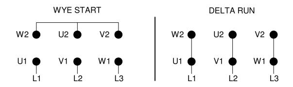
Each motor lead may consist of one or more cables having the same lead marking. To reverse the direction of rotation, interchange line leads L1 & L2, while power is off.
