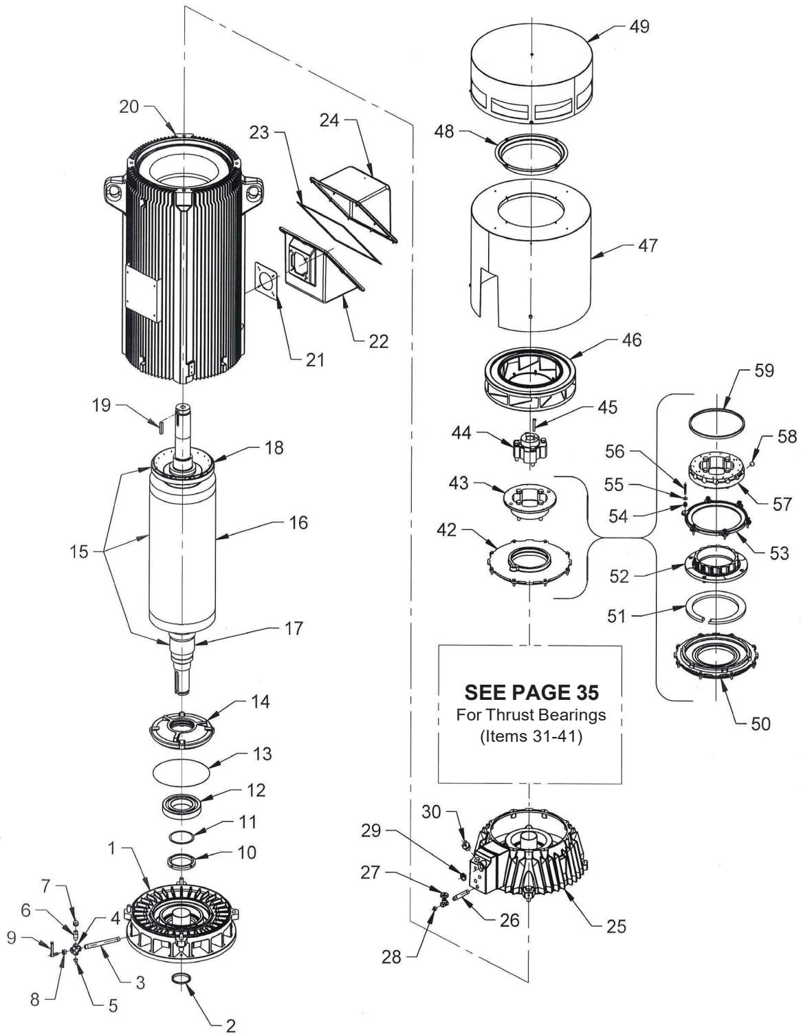
**5812 and 6812 Frame Type JU and JV4****THRUST BEARING DETAILS**
